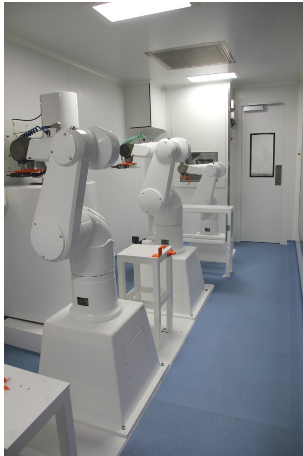
Fig.1. Overview of the robotizic line at TEXERE for production of bone allografts.
